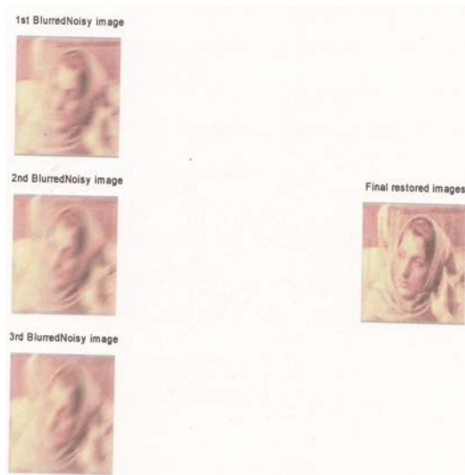
Fig3b: Restored Barbara with ISNR1=2.3492dB for 1 st channel, ISNR2=2.6013 dB for 2 nd channel, ISNR=2.7203dB for 3 rd channel and MSE=393.91
