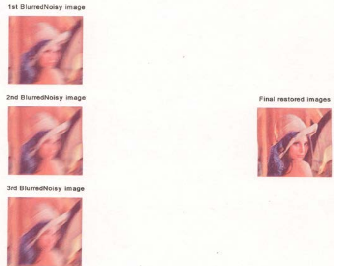
Fig.2b: Restored Lena with ISNR1=5.6260dB for 1 st channel, ISNR2=5.2743dB for 2 nd channel, ISNR3=5.0615dB for 3 rd channel and MSE=189
