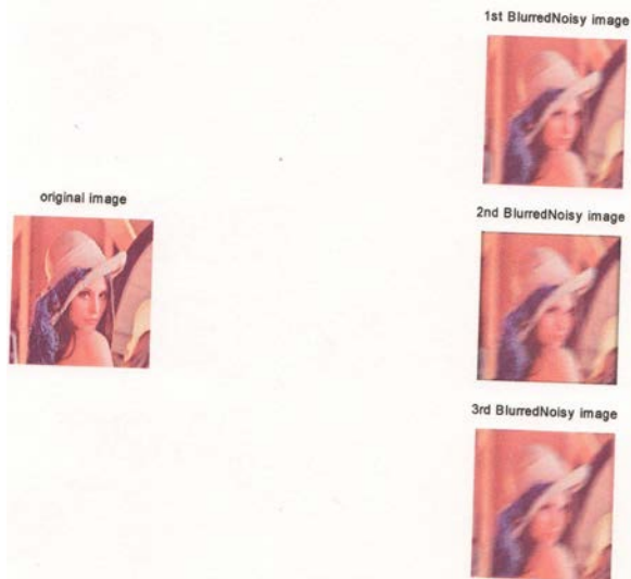
Fig10a: Original Lena using Zonal filter with BSNR1-60dB for 1 st channel, BSNR2-40dB for 2 nd channel and BSNR3-50dB for 3 rd channel at 0.25 Bit Rate.
