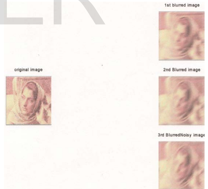
Fig 3a: Original Barbara image with SNR -25dB for 1 st channel, SNR-20 dB for 2 nd channel, SNR=15dB for 3 rd channel
