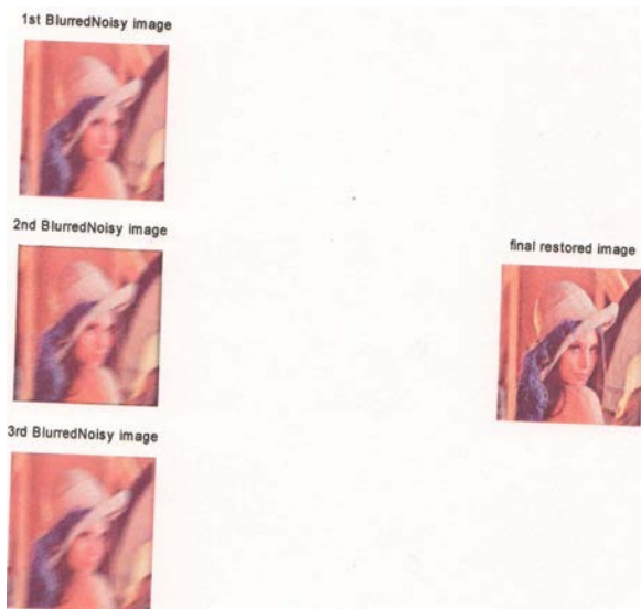
Fig10b: Restored Lena with ISNR1=4.1172dB for 1 st channel, ISNR2=6.3681dB for 2 nd channel and ISNR3=5.0599dB for 3 rd channel and MSE=169.89.
