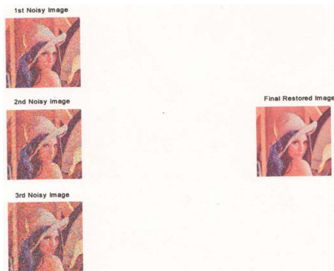
Fig5b: Restored Lena with ISNR1=2,456dB for 1 st channel, ISNR2=3.5840dB for 2 nd channel, ISNR3=4.0231dB for 3 rd channel and MSE=280
