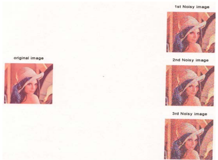
Fig 6a: Original Lena using zonal filter with SNR-25dB for 1 st channel, SNR-20dB for 2 nd channel and SNR-15dB for 3 rd channel at 0.25 Bit Rate
