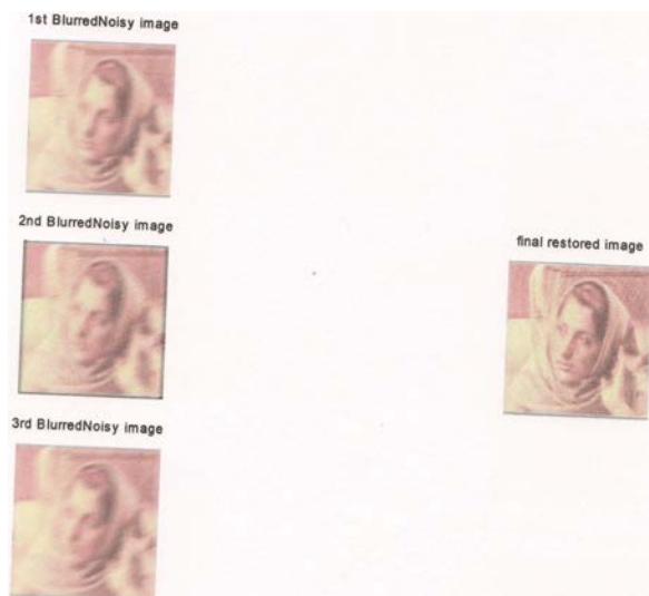
Fig6.1b: Restored Barbara with ISNR1=1.9930dB for 1 st channel, ISNR2=2.8336dB for 2 nd channel and ISNR3=1.5827dB for 3 rd channel and MSE=459.
