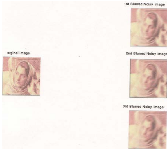
Fig6.3a: original Barbara using zonal filter with BSNR1-60dB for 1 st channel, BSNR2-40dB for 2 nd channel and BSNR3-50dB for 3 rd channel at 0.56 Bit Rate.
