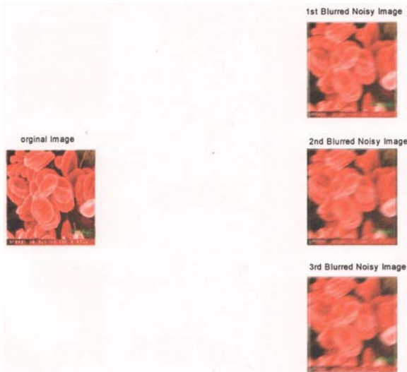
Fig6.7a: Electron Microscopic image of Red Blood Cells using zonal filter with BSNR1-60dB for 1 st channel, BSNR2-40dB for 2 nd channel and BSNR3-50dB for 3 rd channel.
