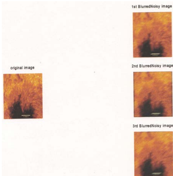
Fig 6.5a: Subspot Image using Zonal filter with BSNR1-60dB for 1st channel, BSNR2-40dB for 2nd channel and BSNR3-50dB for 3rd channel at 0.25 Bit Rate.
