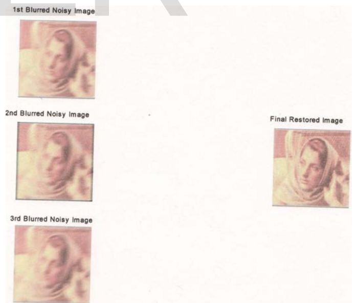
Fig 6.2b: Restored Barbara with ISNR1=1.1857dB for 1 st channel, ISNR2=3.0260dB for 2 nd channel and ISNR3=1.7729dB for 3 rd channel and MSE=439
