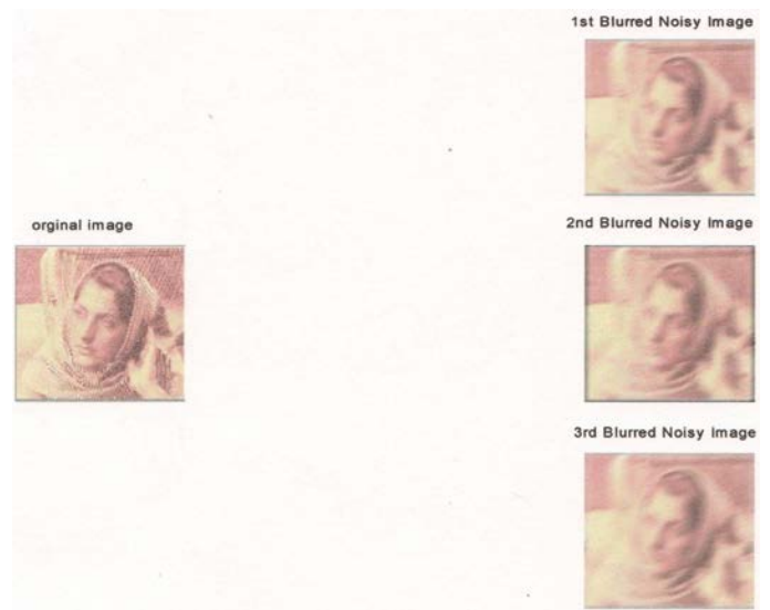
Fig6.2a: original Barbara using zonal filter with BSNR1-60dB for 1 st channel, BSNR2-40dB for 2 nd channel and BSNR3-50dB for 3 rd channel at 0.39 Bit Rate.
