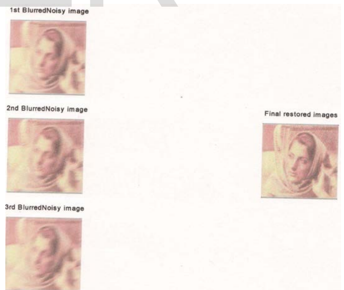
Fig6b: Restored Barbara with ISNR1=1.639dB for 1 st channel, ISNR2=1.2486dB for 2 nd channel and ISNR3=1.2292dB for 3 rd channel and MSE=498.
